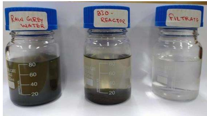
Fig. 12 Physical appearance of raw water, bioreactor treated water and UF filter water
